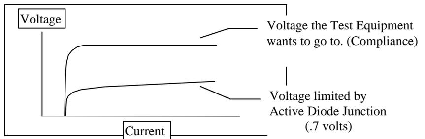
components will actually turn on between .6 - .7 volts. This means that when the tester is trying to learn or test, the active component is turned completely on. Not only does this cause incomplete and erroneous testing, but severe damage to the component can occur. To minimize the risk to the component and to insure accurate testing, the test compliance voltage must be clamped to less than the turn on voltage of the active semiconductor junction.
